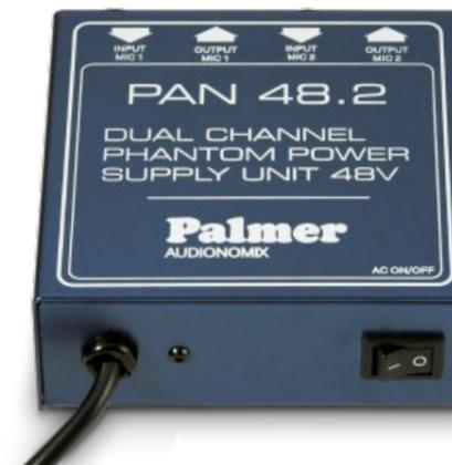
The Palmer PAN48 is a unit for the external power supply of phantom powered appliances. Due to the high current level of a maximum of 20 mA, the application is not just limited to condenser microphones. PAN 48 is excellent for supplying phantom powered active DI-boxes. The box has two channels.
